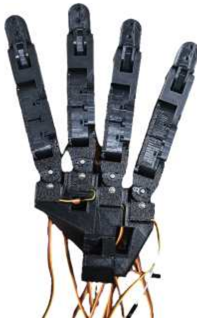
Fig. 13 Intermediate assembly showing the four common finger modules mounted on the palm with the thumb module detached
