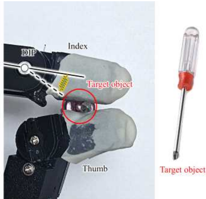
Fig. 11 Fingertip grasp of a thin object enabled by the passive fingertip mechanism
