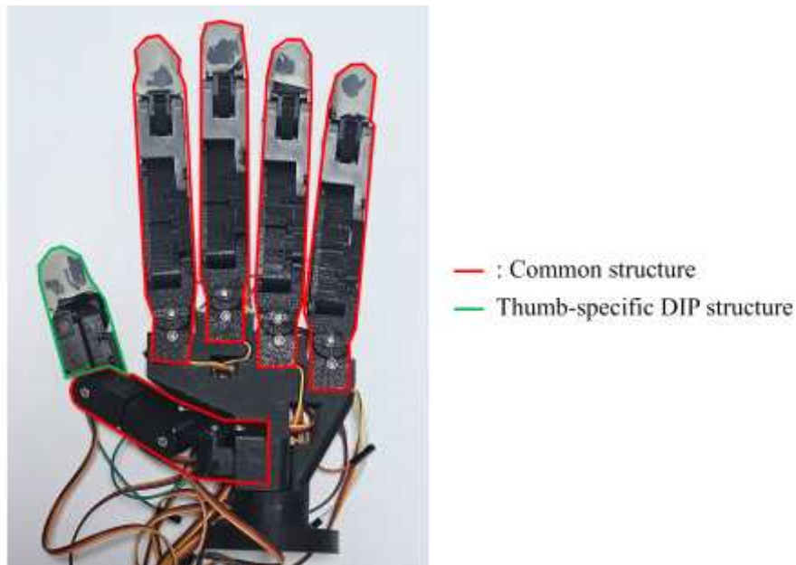
Fig. 12 Modular finger arrangement on the palm: common finger modules (index to little finger) and thumb-specific DIP part
